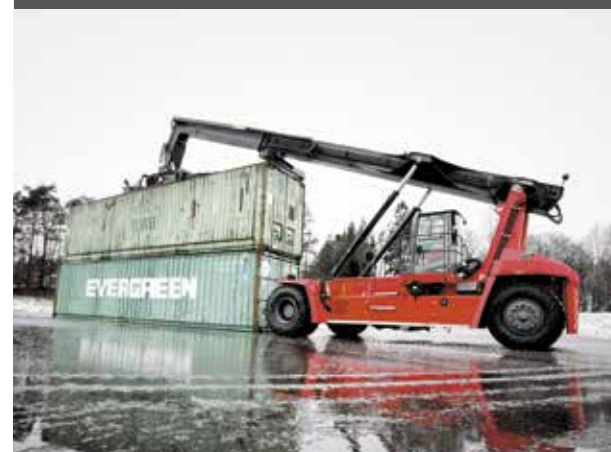
Precise lifting of long container end-on - 40 ft
